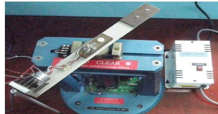
Figure 3.7: Test model of rotary inverted pendulum Kri PP-300 at the Measuring – Control Laboratory, Thai Nguyen University of Technology
