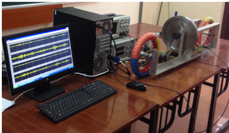
Fig 4.16. Experimental control table of self-balancing two-wheeled bicycle
